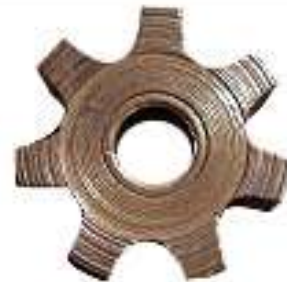
Figure 2: An idler with wear from large Abrasive particulate
