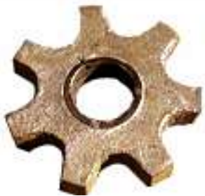
Figure 1: An idler with Corrosive wear
